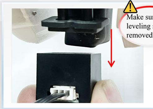
Make sure the leveling switch is removed!
