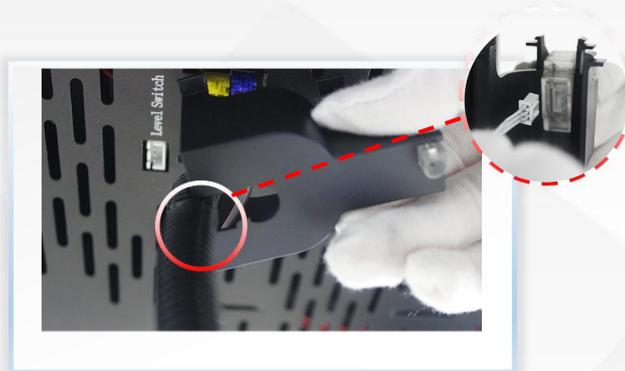
Take out the filament detection sensor, connect the filament detector wire. Snap the bellows into the bracket slot.
