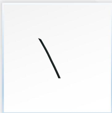
1. Use diagonal pliers to cut the filament at an angle of 45° .
