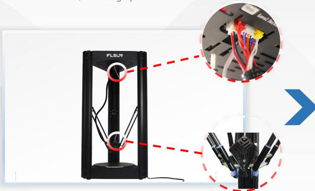
Install the effector module with the extruder hood facing forward. Plug the cable into the top shell adapter board, the color of the connectors is corresponding.
