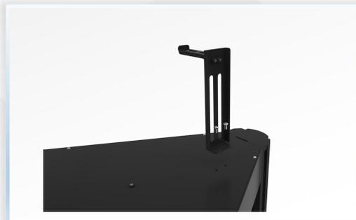
Install the filament holder on the top of the printer, paying attention to the installation direction.
