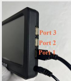
Connect the PAD's **port 1** and the printer, Take out the adapter and power on the PAD.
