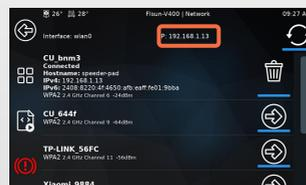
Click "Configuration>Network" to connect to wifi. After the connection is successful, an IP address is generated, and it can be entered into the browser to realize online printing.
